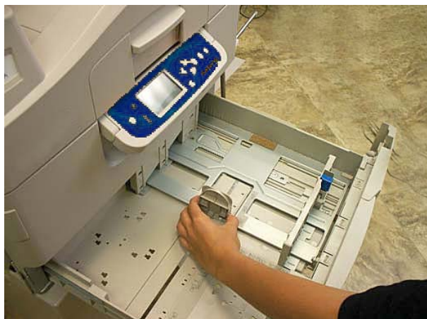
Adjust Rear Stopper tab
