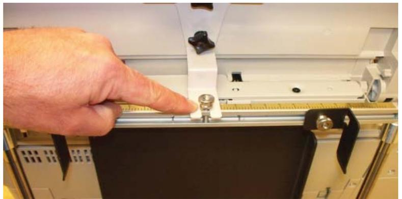
After Adjusting the Feeder height and the Printer Stand height the plastic sensor block on the back of the Media Guide Plate should be positioned as shown. Correct positioning is critical to activating the Feeder Present Sensor on the printer. Raise the two outside leveling guides to tilt the feeder into the printer, depressing the Presence sensor.
