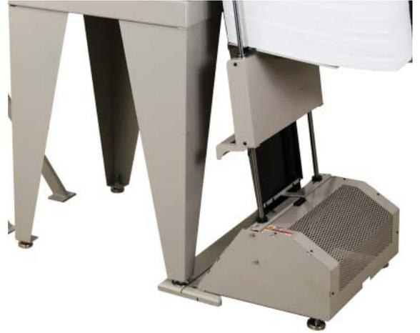
Align the top of the Feeder's Media Guide Plate with the red lines as shown. Adjust the feeder using the adjustable slide guides on the bottom.
