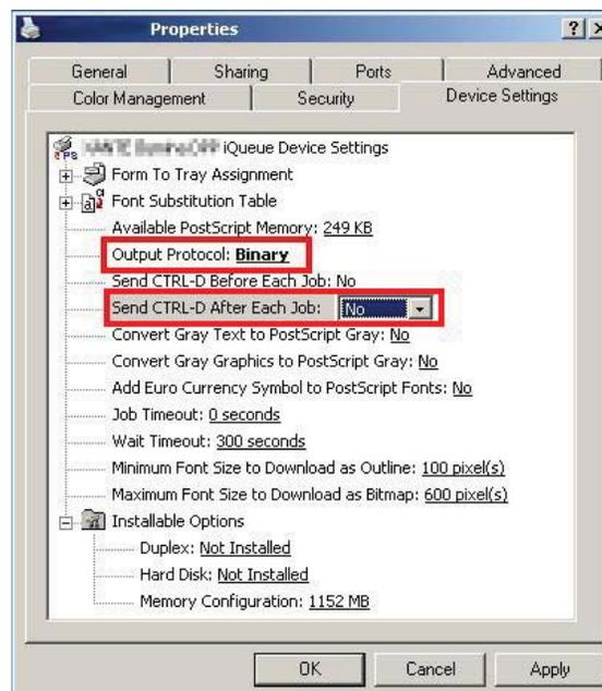
Change the Output Protocol to Binary and the Send CTRL-D After Each Job to No as shown above. Click OK to complete iQueue and Printer driver installation.
