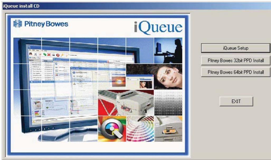
Once iQueue is installed, launch iQueue to identify the computers IP Address. This address is needed for the iQueue print driver installation. If your computer has more than one Ethernet card installed you will see two IP Addresses. Select the primary IP Address for the printer installation. Consult your system administrator if you are unsure about what IP Address to use.
